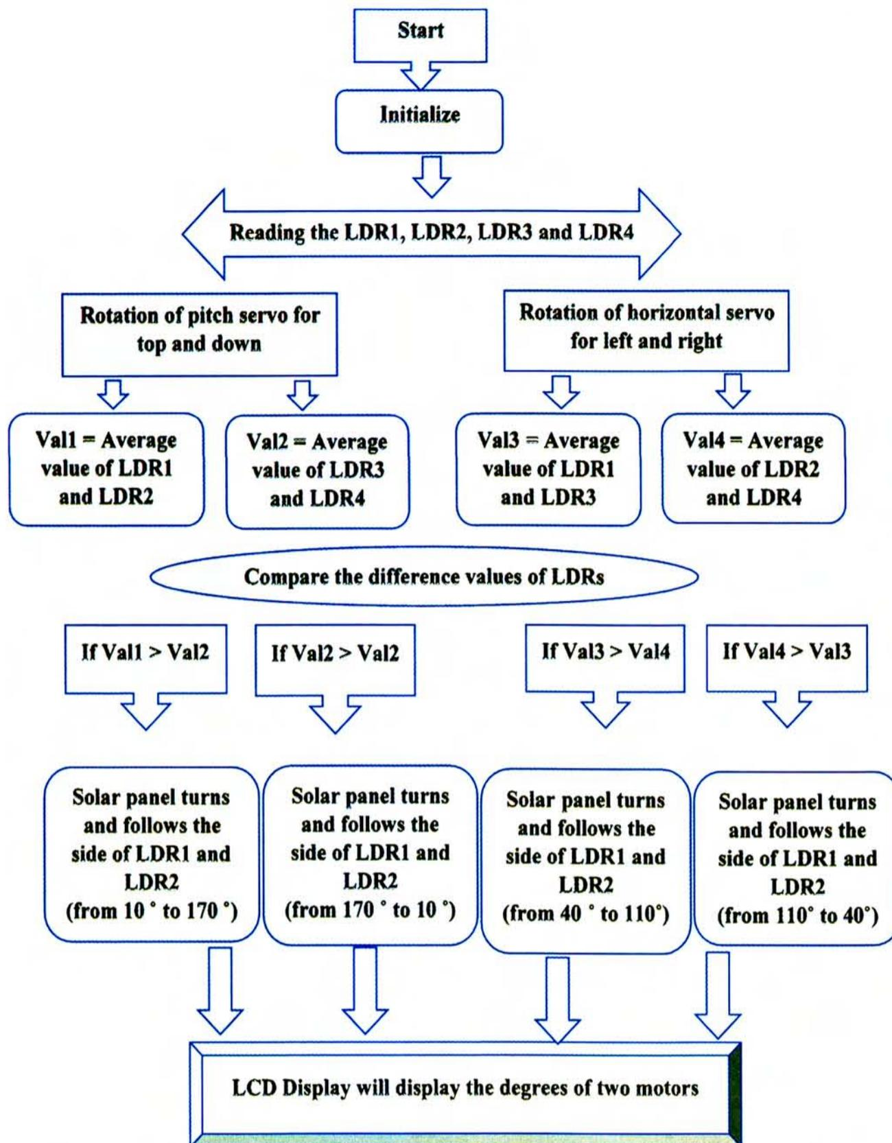
Figure 5. Software procedure of prototype dual axis solar tracker
